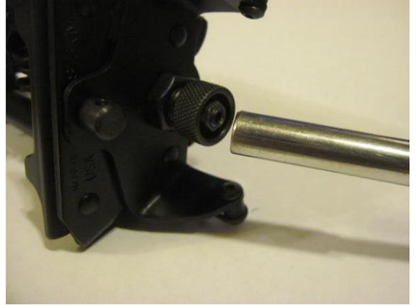
Before removing the knurled lockdown nut, invert the body of the bipod and locate the pivot rod retaining pin. This is a cross pin that keeps the threaded pivot rod from rotating. During the next steps, you will need to hold the pivot rod and cross pin in place with your finger to keep it from sliding out and shifting out of position.
