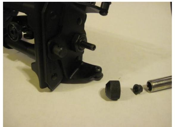
Place the spacer over the threaded pivot rod, and install the handle. The handle can be "parked" without affecting the pivot tension by pulling it directly back from the bipod and rotating it to the desired position. It is spring loaded and will reengage the lock when released. A screw head is visible on the lever assembly. DO NOT attempt to adjust this screw! This screw holds the parts of the lever together and is not adjustable.
